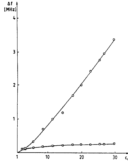
Figure 3. Changes in resonance frequencies as a function of the dielectric constant (○) even mode, (□) odd mode. Measurements have been made with paper and different plastics. Frequency changes correspond to 0.1 mm thick layers.
